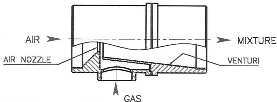
Despite the atmospheric mixers, the pressure of the mixture in this type of mixers is considerable and continuous pressure shall make a flame with a high temperature at the burner head as well as the object to be heated.
