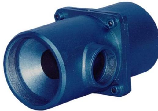
Despite the atmospheric mixers, this type of mixer does not require the high-pressure of air or gas. The required pressure for injecting gas in the burner is secured by a Zero-governor. The pressure of the required air varies from 20 to 110mbar.
