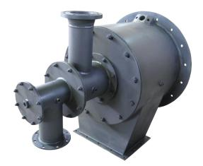
This burner has provision for gas pilot and ultraviolet flame supervision device. Both gas and oil flames are tile – stable over a fairly wide range of air/fuel ratios. The burner can be used in cold sealed-in combustion chambers with light oil or gas.
