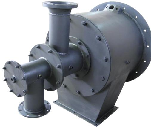
This burner has provision for gas pilot and ultraviolet flame supervision device. Both gas and oil flames are stable – stable over a fairly wide range of air/fuel ratios. The burner can be used in cold sealed-in combustion chambers with light oil or gas.
