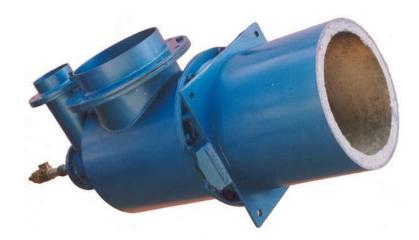
This burner has provision for gas pilot and ultraviolet flame supervision device . Both gas and oil flames are tile – stable over a fairly wide range of air /fuel ratios . The burner can be used in cold sealed-in combustion chambers with light oil or gas .
