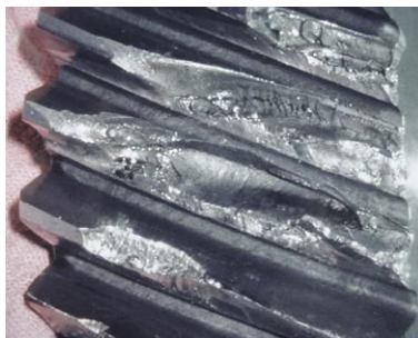
Fig. 2. Gear teeth torn away from the gear surface
