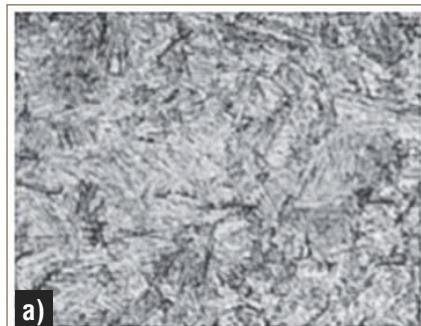
Fig. 9. Core microstructure variation due to quenching: (a) fully martensitic microstructure with a core hardness of 44 HRC, (b) martensitic microstructure with transformation products (bainite and ferrite) present with a core hardness of 26 HRC
