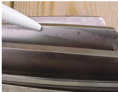
Fig. 4. Soft spots in the carburized case (observed after shot peening)
