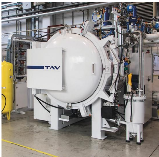
Fig. 1. Vacuum sintering furnace (T 50-50-75) with water-cooled binder trap
