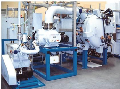
A sintering furnace that utilizes Pfeiffer Vacuum rotary vane pumps, Roots blowers and leak detection equipment.
