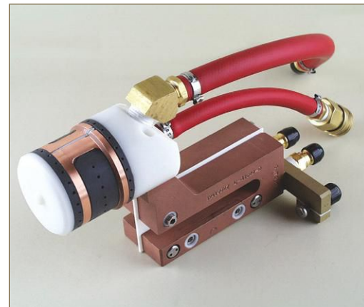
Fig. 7. Single-shot inductor with machined integral quench
