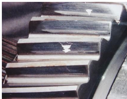
Fig. 6. Inclusion-initiated pitting in vacuum-degassed steel
