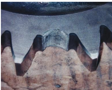
Fig. 1. Tooth breakage due to bending fatigue
