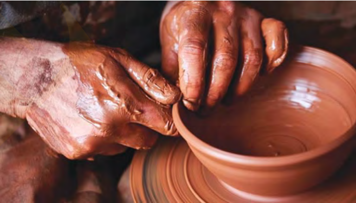
Fig. 2. Modeling produces a useful shape from a raw lump of clay but requires energy inputs from human labor and an electric motor.
