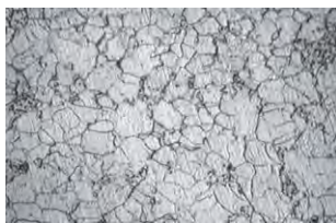
Fig. 8. Cross section from the furnace chamber. Steel grade 16Mo3, ferrite-carbide structure, separation of carbides on grain boundaries, ASTM Grain No. 10, hardness 126 HV10, 500X, 2% Nital
