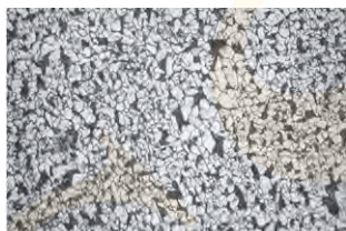
Fig. 5. Cross section from the side embedded in the brick wall. Steel grade 16Mo3, ferrite/pearlite microstructure, ASTM grain No. 10, hardness 148 HV10, 100X, 2% Nital
