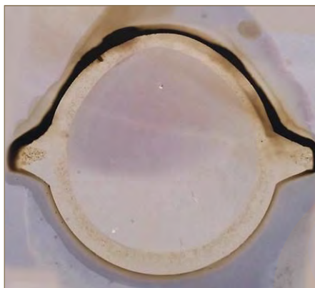
Fig. 4. Baumann micrographic examination for the presence of sulfur
