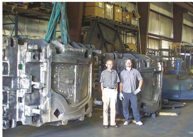
Fig. 6. Automotive stamping dies made of cast iron after plasma/ion nitriding (courtesy of Advanced Heat Treat Corp.)
