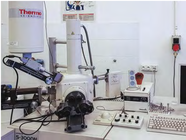
Fig. 2. Scanning electron microscope (equipped with attachments for determination of chemical composition in micro-areas and phase identification via the EBSD method)
