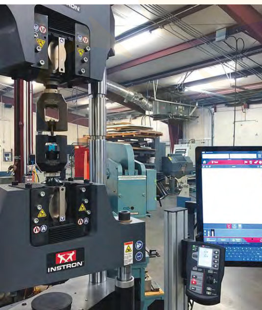
Fig. 1. Universal testing machine in the configuration for tensile testing of bolts
