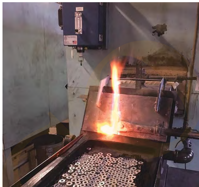
Fig. 2. An atmosphere furnace heat treating parts to adjust their hardness and improve appearance.
