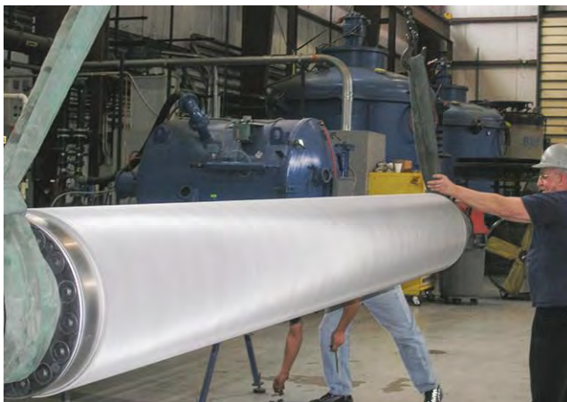
Fig. 5. Engraved embossing roll after plasma/ion nitriding (courtesy of Advanced Heat Treat Corp.)
