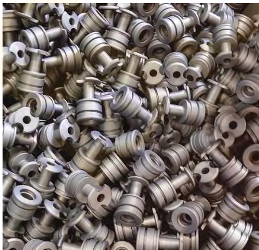
Fig. 7. Components of the pneumatic system after gas nitriding (courtesy of Advanced Heat Treat Corp.)
