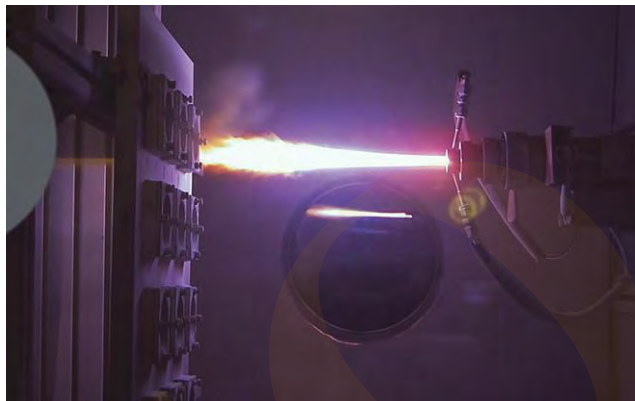
Fig. 3. Thermal spray applying a coating to improve part performance in service.
