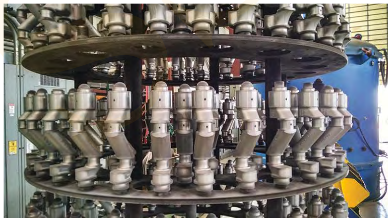
Fig. 4. Lot of compressor crankshafts after ion/plasma nitriding. Note mechanical masking with the ball bearings on top of the parts (courtesy of Advanced Heat Treat Corp.).
