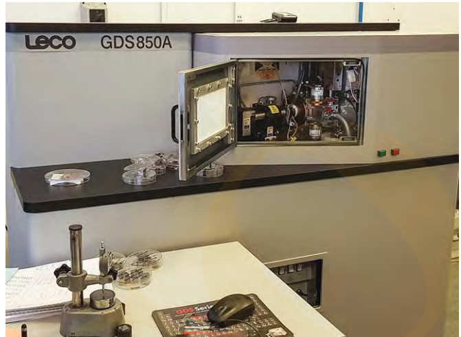
Fig. 3. Optical glow-discharge atomic-emission spectrometer for studying chemical composition of metals and ceramics
