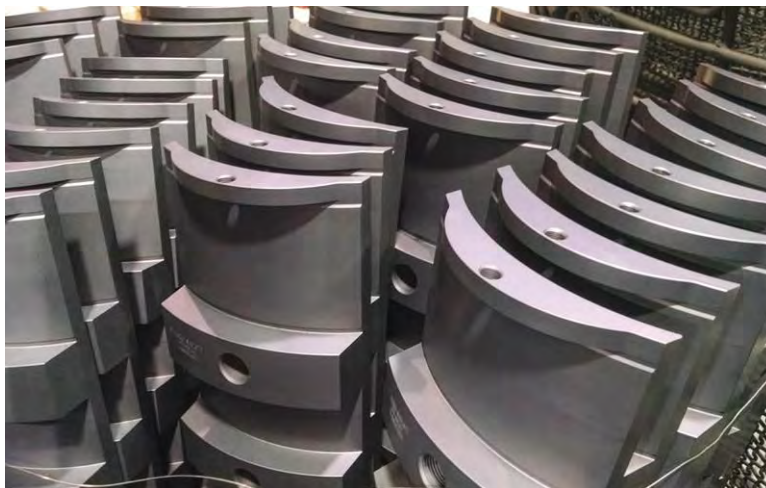
Fig. 8. Slides for oil-and-gas machines after UltraOx gas processing (courtesy of Advanced Heat Treat Corp.)
