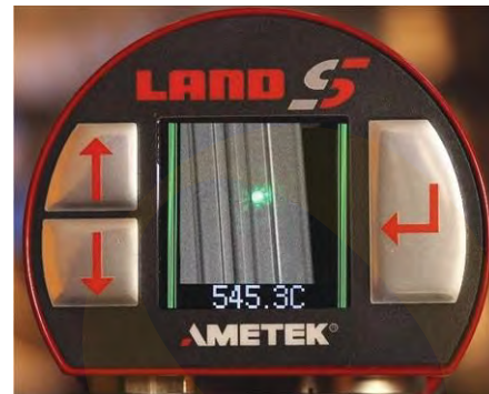
Fig. 4. Pyrometer image view of the target with LED illuminated
