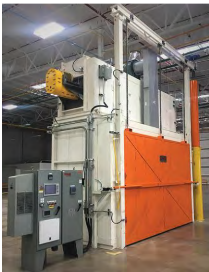
Fig. 2. Oven design includes supply plenums installed on both sides of the work chamber with the return plenum mounted on the ceiling of the work chamber.
