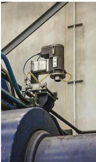
Fig. 5. SPOT AL EQS with actuator above the press exit
