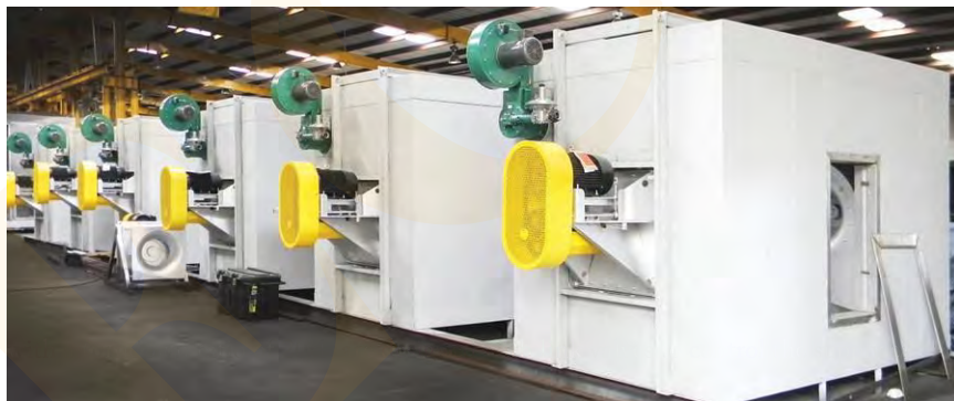
Fig. 4. Coil-coating continuous-oven system
