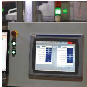
Fig. 3. Digital outputs from the SPOT AL EQS pyrometers allow them to be integrated into control systems
