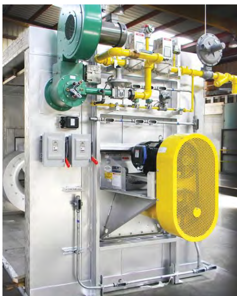
Fig. 5. Coil-coating oven combustion chamber
