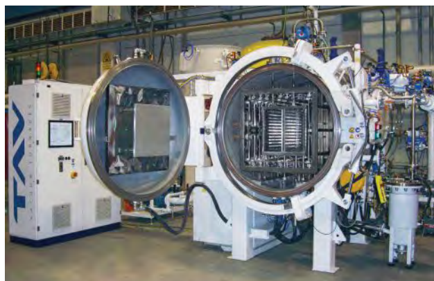
Fig. 2. Open sintering furnace (courtesy TAV VACUUM FURNACES)
