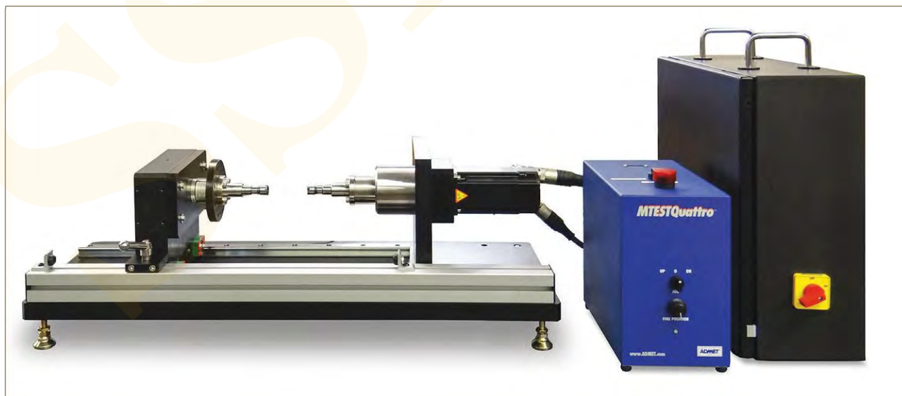
Fig. 9. A torsion fatigue testing system configured for performing fatigue tests on small components used in portable electronic equipment (courtesy ADMET).
