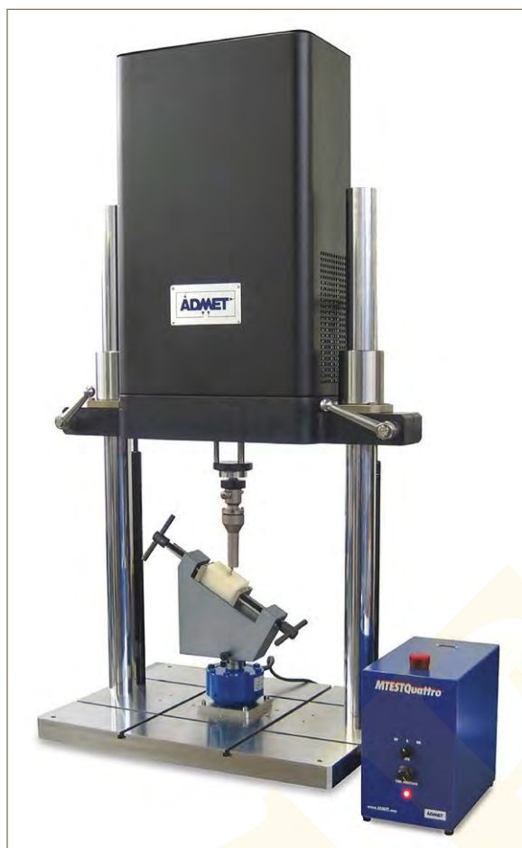
Fig. 8. This fatigue testing system is configured for testing dental implants according to ISO 14801 Dentistry Implants – Dynamic Fatigue Test for Endosseous Dental Implants (courtesy ADMET).
