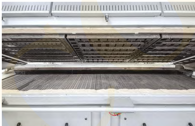
Fig. 2. Furnace interior with different air-guidance systems depending on the different heating zones
