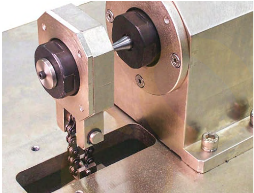
Fig. 7. Ducom Instruments rotating-bar bending fatigue-testing machine. A test piece mounted as a cantilever with single-point loading is made to rotate and thus subjected to a bending moment. Principle is similar to Wohler's machine built in the 1800s (courtesy of Ducom Instruments)
