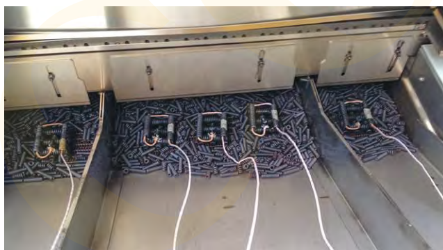
Fig. 3. Measurement setup for temperature uniformity survey with bulked load separated in three lanes
