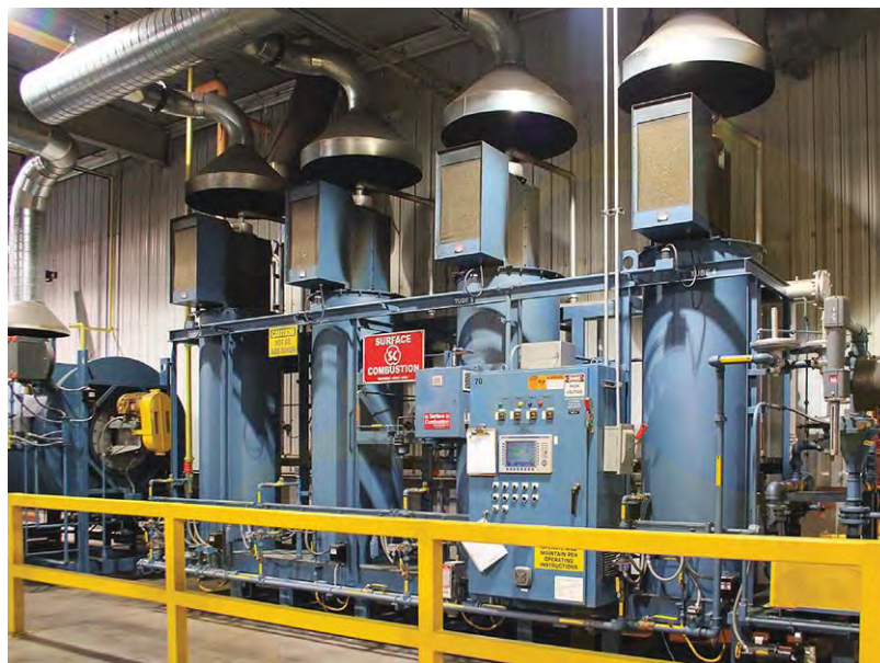
Fig. 3. Modular multi-retort endothermic gas (Rx®) generator (courtesy of Surface Combustion, Inc.)
