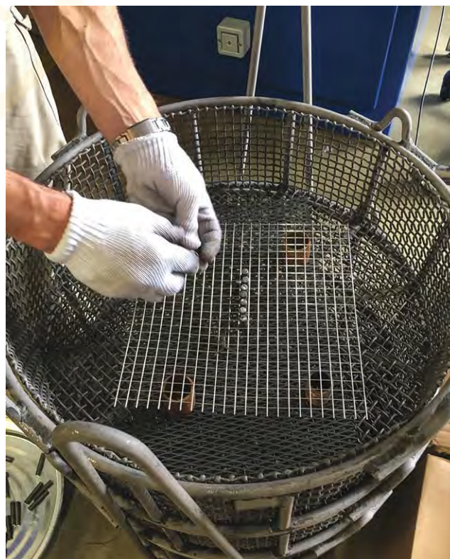
Fig. 4. Two sets of FNC test parts run in a sealed pit furnace with an ammonia, nitrogen and \text{CO}_2 atmosphere.
