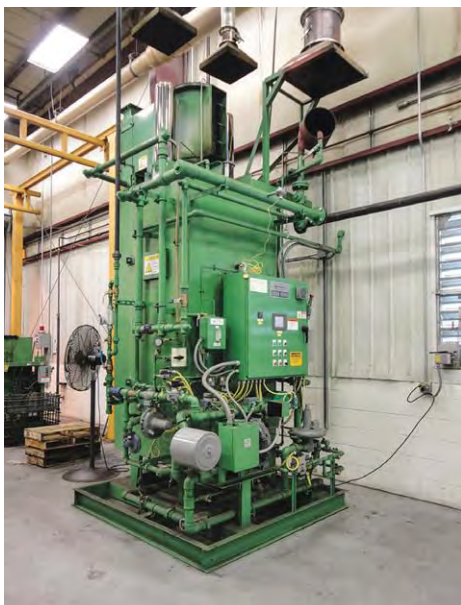
Fig. 2. Single-retort endothermic gas generator (courtesy of AFC-Holcroft)
