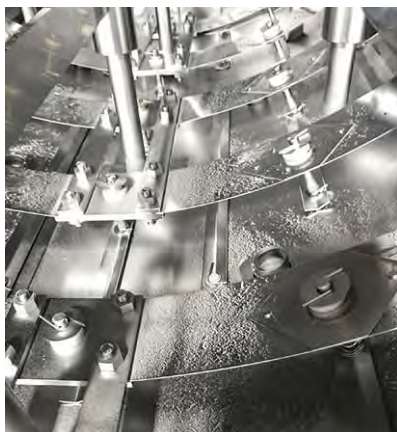
Fig. 3. Titanium powder spewed and fused to molybdenum heating elements
