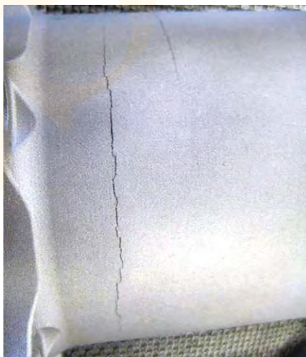
Fig. 5. Crack due to improper match of printed cross section vs. build thickness
