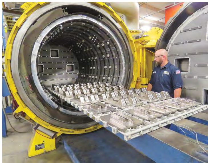
Fig. 2. Vital equipment needed for additive manufacturing: the vacuum furnace
