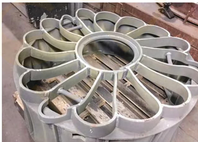
Fig. 3. Daisy-wheel fixture – a round shaft would go through the center and either be welded to a plate below or directly to the groove in the center.
