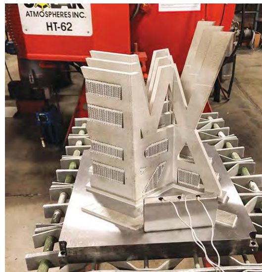
Fig. 6. Never thermocouple the build plate itself
