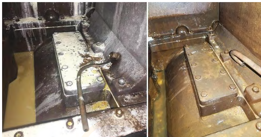
Fig. 4. Internal views of a contaminated pump vs. a clean pump
