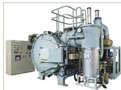
Fig. 3. A single-chamber batch vacuum heating furnace
