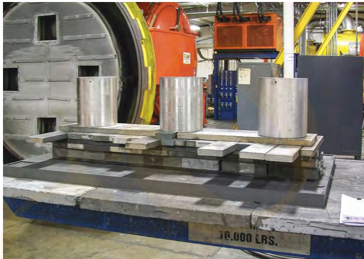
Fig. 7. Weights strategically placed and used to creep flatten build plate
