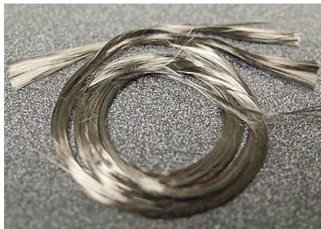
Fig. 1. Typical carbon fibers used in making C/C fixturing (courtesy of Acriss USA)
