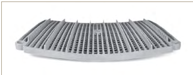
Fig. 2. This 66-pound (30-kg) grid showed significant distortion after nine months of furnace heating/cooling, with no intermediate straightening attempted during that time (courtesy of Schunk Graphite).
