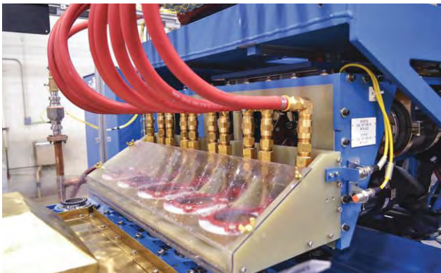
Fig. 6. Modular coil bank enables coil-to-part consistency
