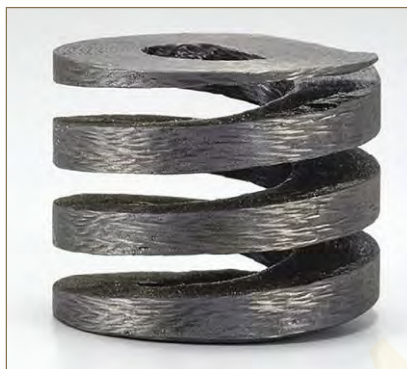
Fig. 6. C/C coil spring (courtesy of Across USA)
