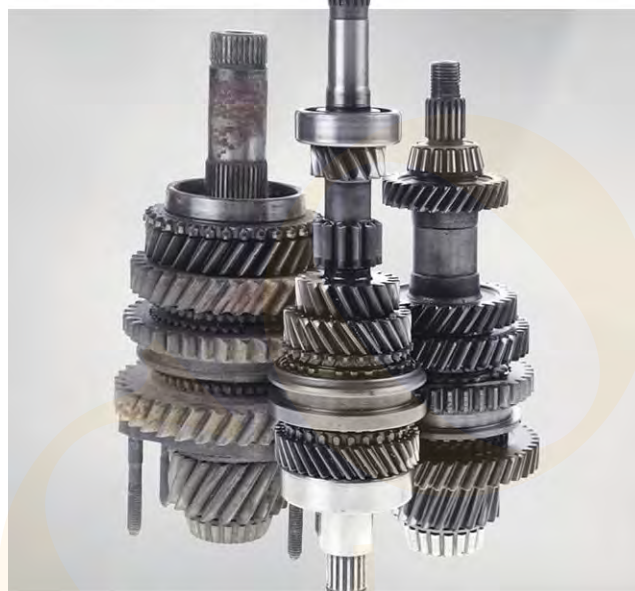
Fig. 3. Dematerialization over decades has resulted in the lighter, therefore more fuel-efficient, foreground part
