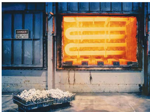
Fig. 5. A real-world radiant-tube application. One can visually notice areas in the tube glowing brighter than others, indicating temperature non-uniformity.
