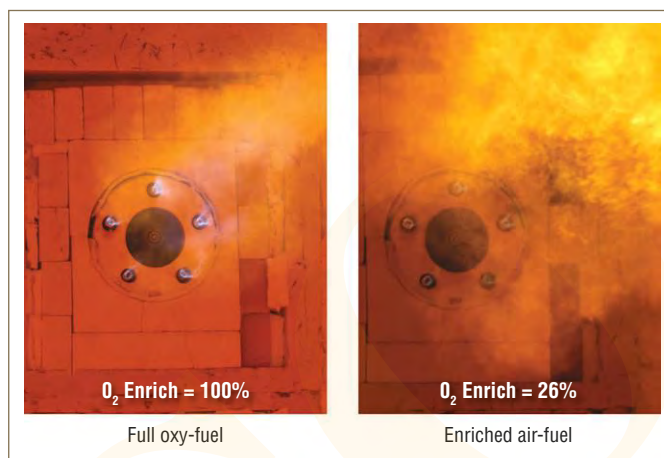
Fig. 3. Range of oxygen-enrichment operation of TEB technology
