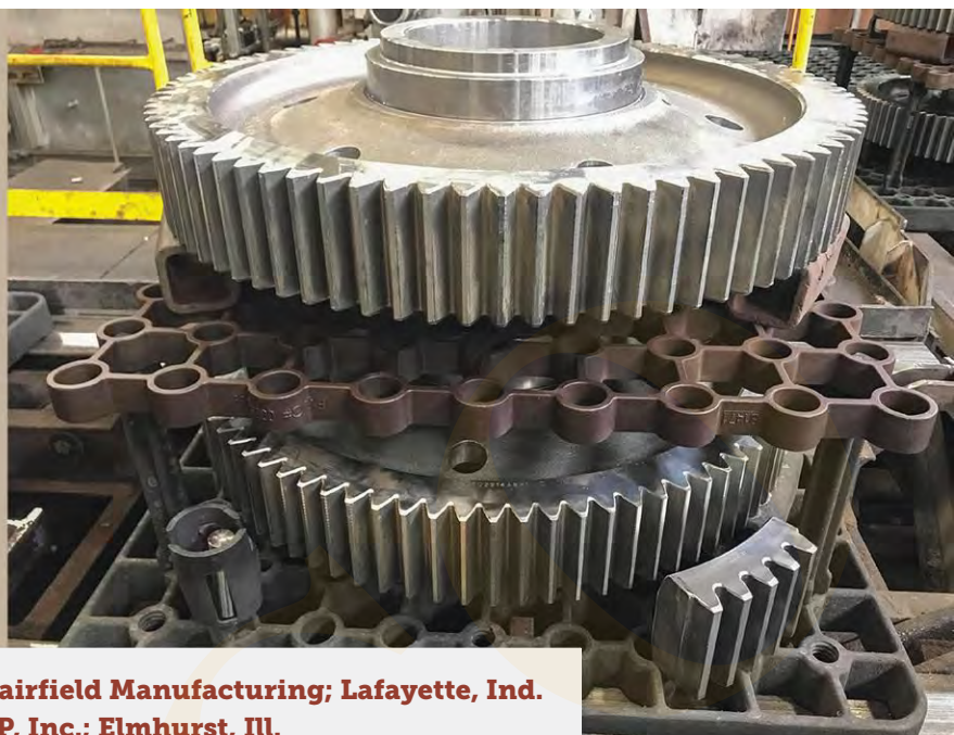
Fig. 2. Carburized bull gear
