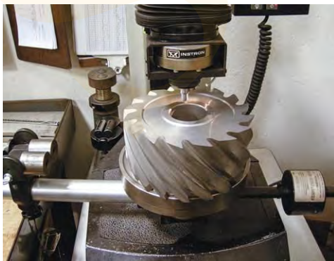
Fig. 1. Fixed-location indentation-style bench hardness tester
