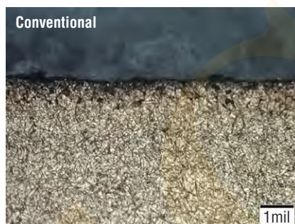
Fig. 5. Flank (midpoint) comparisons performed on tooth #2 of the bull gear from both facilities [4]
