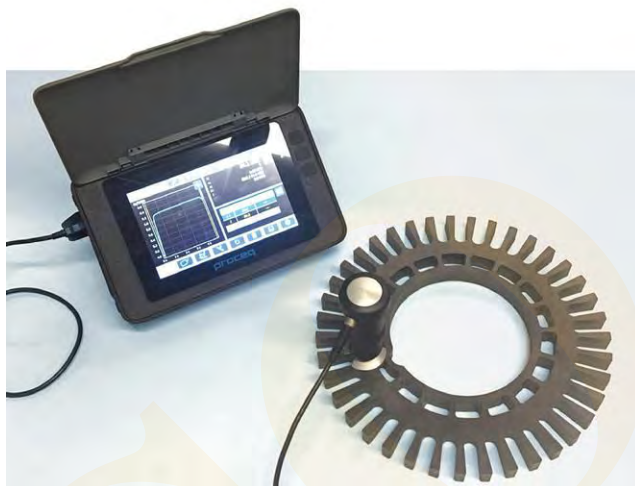
Fig. 2. Portable dynamic rebound-style hardness tester (courtesy of Columbia Machine Inc.)
