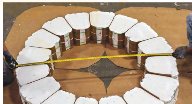
Shop layout of new hot-face Z-Blok2 trapezoidal folded modules for retort ring
