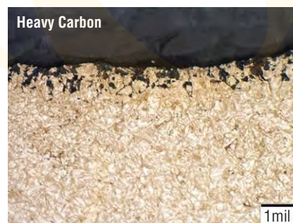
Fig. 5. Flank (midpoint) comparisons performed on tooth #2 of the bull gear from both facilities [4]
