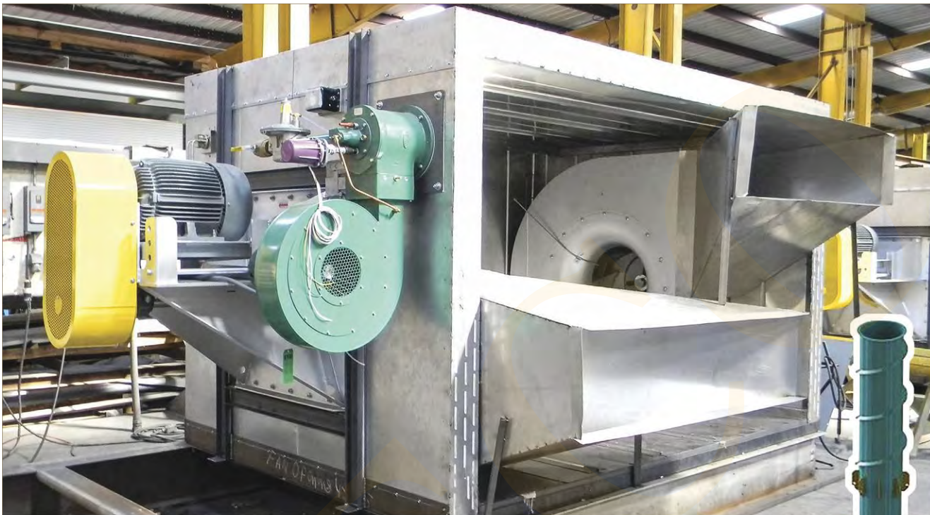
Fig. 3. The rendering shows the design of a recuperative thermal oxidizer for an aluminum parts producer. The oxidizer is part of an integrated melt system being provided by a metals-recovery systems house.
