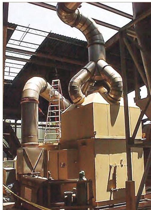
Fig. 2. This custom-engineered configuration, which includes a thermal oxidizer equipped with a quad-downflow inlet plenum, axial-mounted down-fired burner and primary and secondary heat exchangers, maximized turbulence in the combustion chamber. This resulted in good destruction efficiency and protected the burner from potential particulate carryover.
