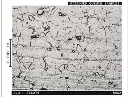
Fig. 6. Inco 718 solution annealed and nitrogen quenched (500X)
