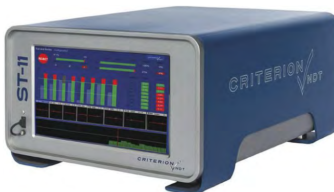
Fig. 2. Modern eddy current testing instrument with touch-screen display showing results of multi-frequency testing
